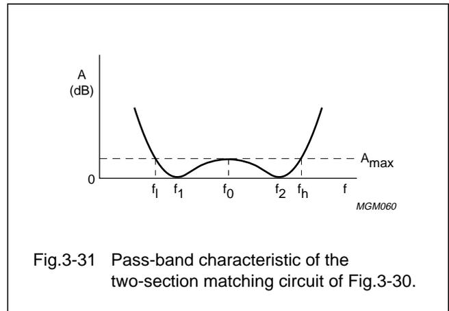
Fig.3-31 Pass-band characteristic of the two-section matching circuit of Fig.3-30.
