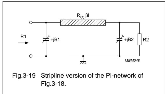
Fig.3-19 Stripline version of the Pi-network of Fig.3-18.
