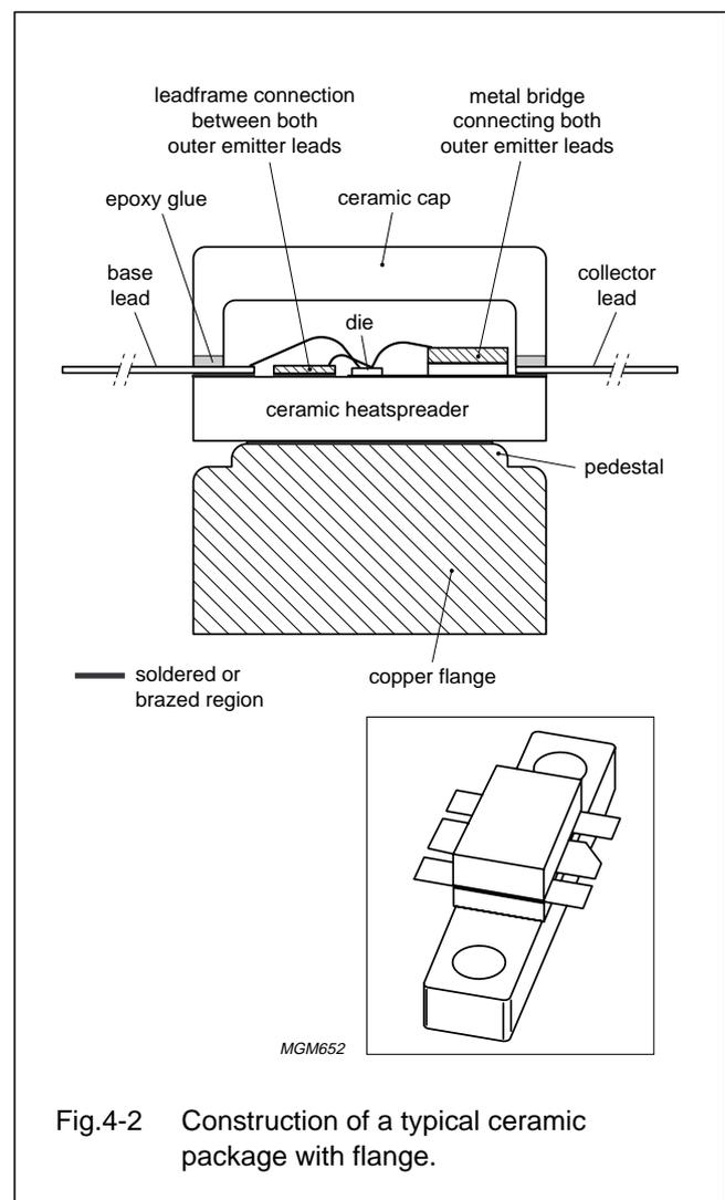
Fig.4-2 Construction of a typical ceramic package with flange.
