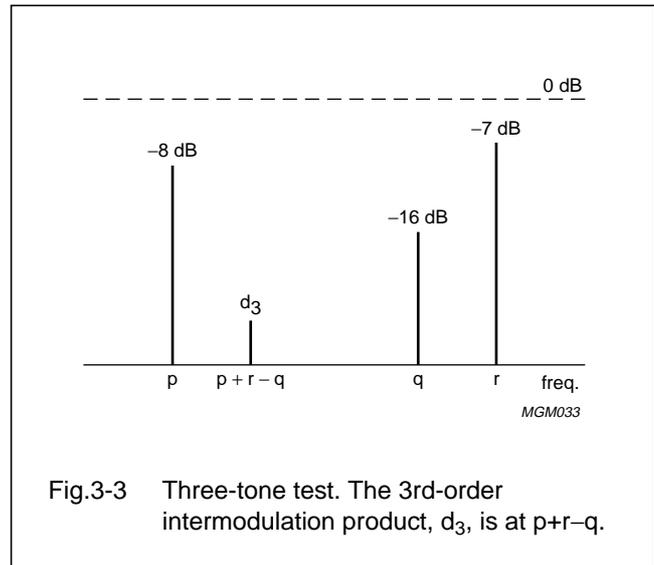
Fig.3-3 Three-tone test. The 3rd-order intermodulation product,  $d_3$ , is at  $p+r-q$ .
