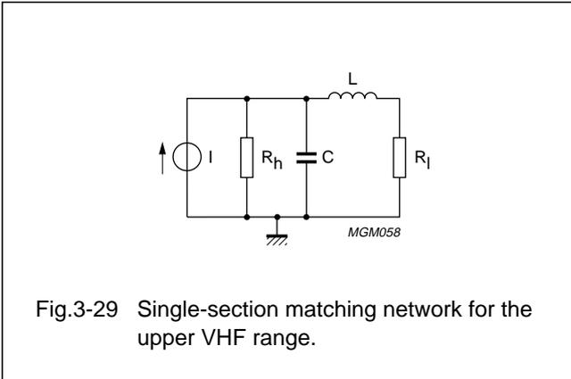
Fig.3-29 Single-section matching network for the upper VHF range.
