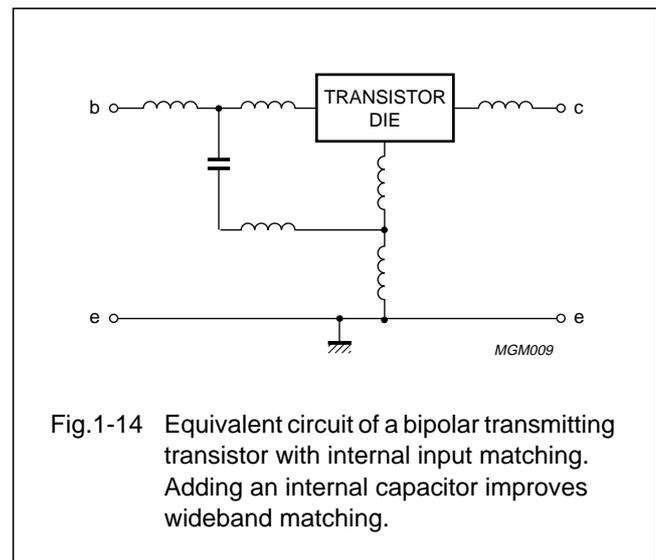
RF transmitting transistor and power amplifier fundamentals
