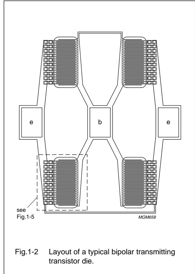
Fig.1-2 Layout of a typical bipolar transmitting transistor die.
