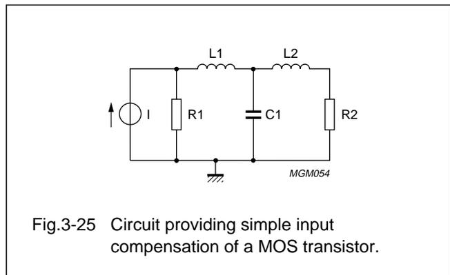
Fig.3-25 Circuit providing simple input compensation of a MOS transistor.
