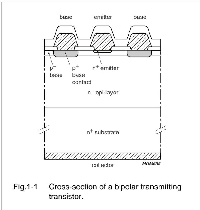
Fig.1-1 Cross-section of a bipolar transmitting transistor.
