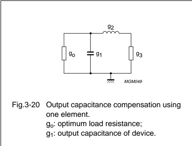
In the circuit of Fig.3-20, the filter elements are:
