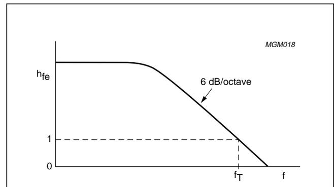
Fig.2-5 RF current gain,  $h_{fe}$  as a function of frequency.  $f_T$  is the transition frequency.
