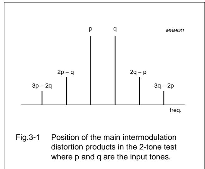
Fig.3-1 Position of the main intermodulation distortion products in the 2-tone test where  $p$  and  $q$  are the input tones.
