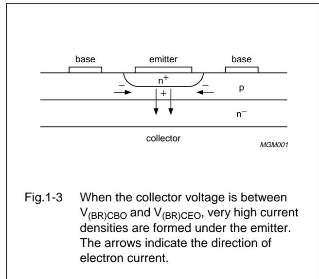
Fig.1-3 When the collector voltage is between  $V_{(BR)CBO}$  and  $V_{(BR)CEO}$ , very high current densities are formed under the emitter. The arrows indicate the direction of electron current.
