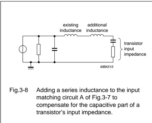
Fig.3-8 Adding a series inductance to the input matching circuit A of Fig.3-7 to compensate for the capacitive part of a transistor's input impedance.
