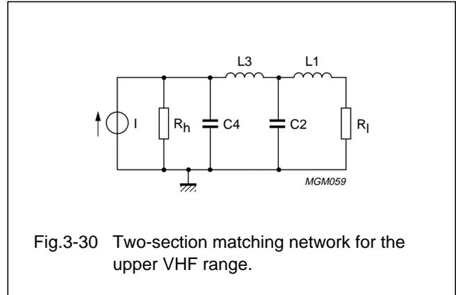
Fig.3-30 Two-section matching network for the upper VHF range.
