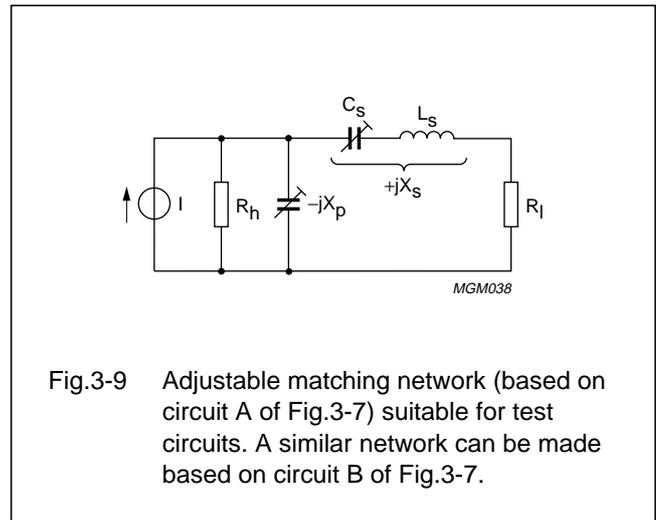
Fig.3-9 Adjustable matching network (based on circuit A of Fig.3-7) suitable for test circuits. A similar network can be made based on circuit B of Fig.3-7.
