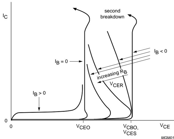
Fig.2-2 Definition of breakdown voltages.
