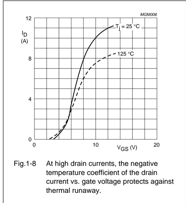
Fig.1-8 At high drain currents, the negative temperature coefficient of the drain current vs. gate voltage protects against thermal runaway.
