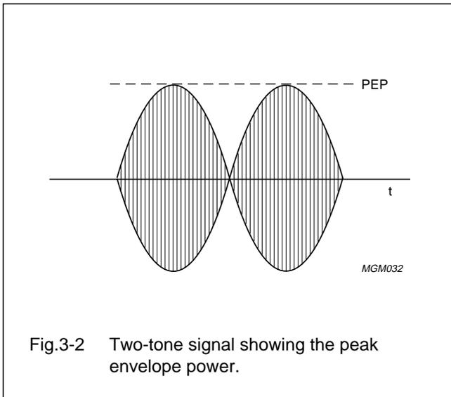
Fig.3-2 Two-tone signal showing the peak envelope power.
