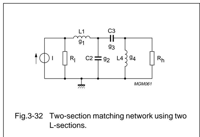
Fig.3-32 Two-section matching network using two L-sections.
