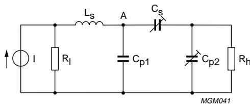
Fig.3-12 Matching network formed by combining those shown in Figs.3-9 and 3-10.
