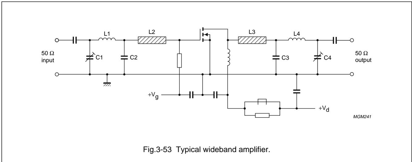
Fig.3-53 Typical wideband amplifier.
