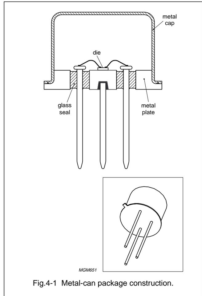
Fig.4-1 Metal-can package construction.
