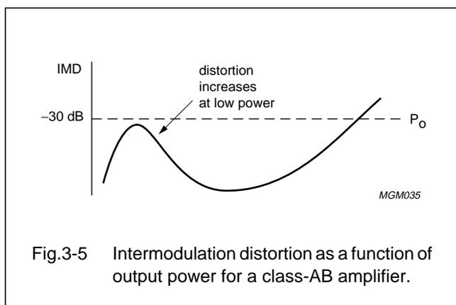
The increasing distortion at low powers is due to 'cross-over' distortion, i.e., distortion during the transition from class-A to class-B operation.
