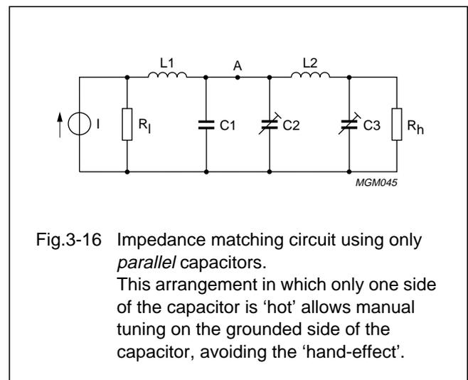
Fig.3-16 Impedance matching circuit using only parallel capacitors. This arrangement in which only one side of the capacitor is 'hot' allows manual tuning on the grounded side of the capacitor, avoiding the 'hand-effect'.
