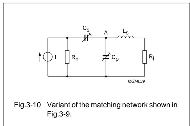
Fig.3-10 Variant of the matching network shown in Fig.3-9.
