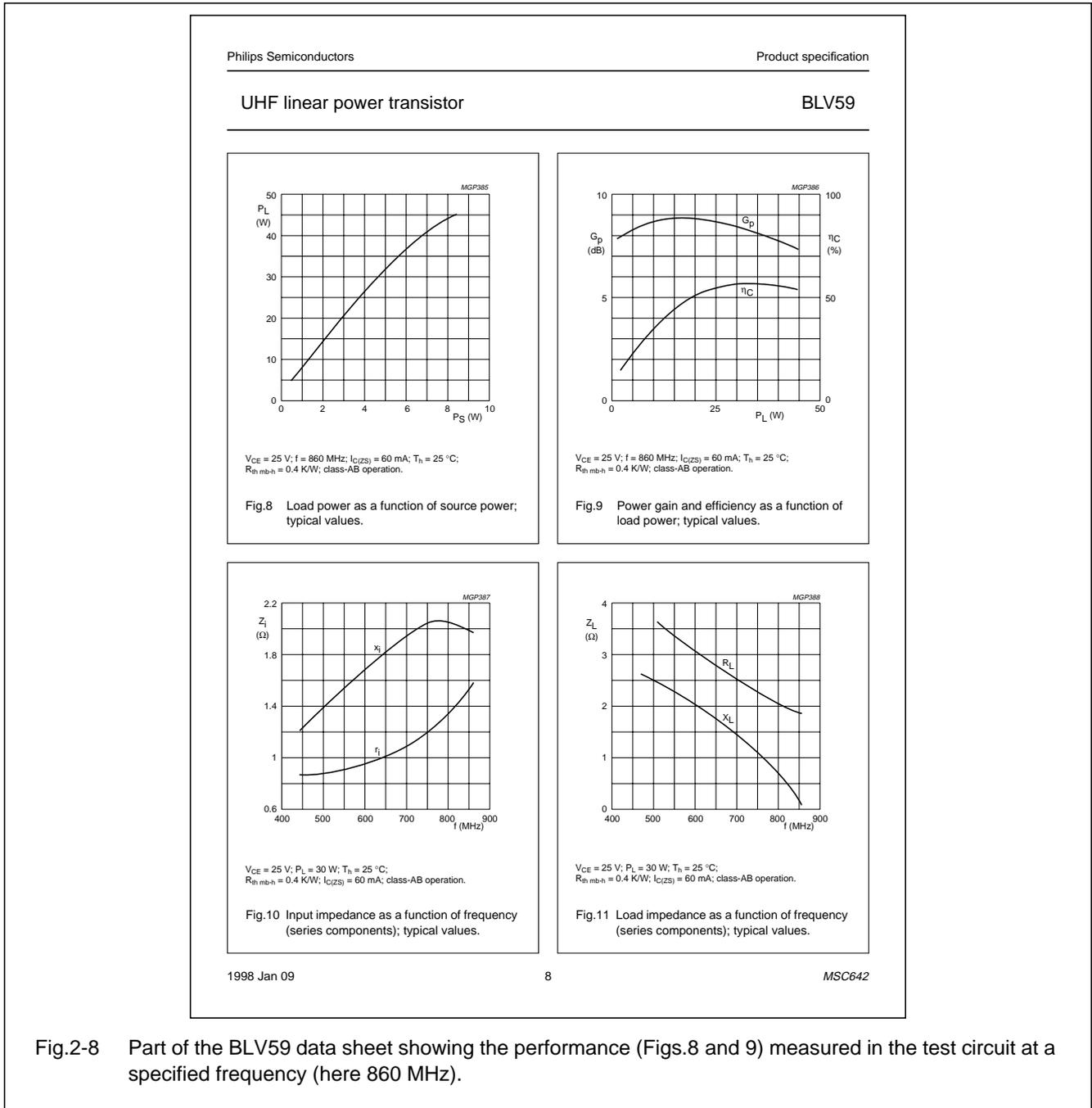
Fig.2-8 Part of the BLV59 data sheet showing the performance (Figs.8 and 9) measured in the test circuit at a specified frequency (here 860 MHz).
