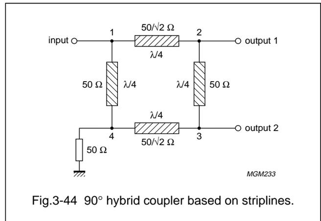
Fig.3-44 90° hybrid coupler based on striplines.
