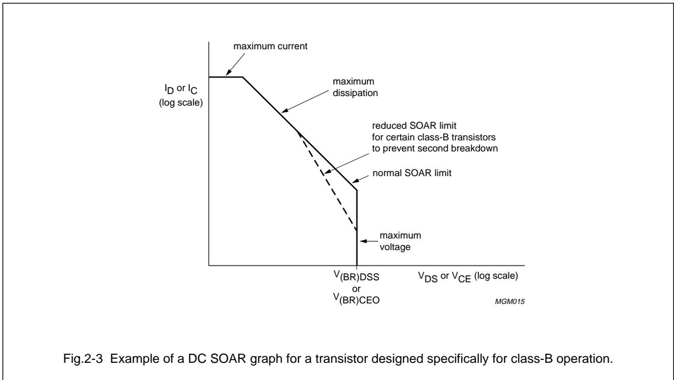
Fig.2-3 Example of a DC SOAR graph for a transistor designed specifically for class-B operation.
