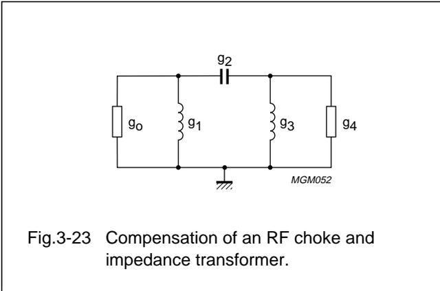
Fig.3-23 Compensation of an RF choke and impedance transformer.
