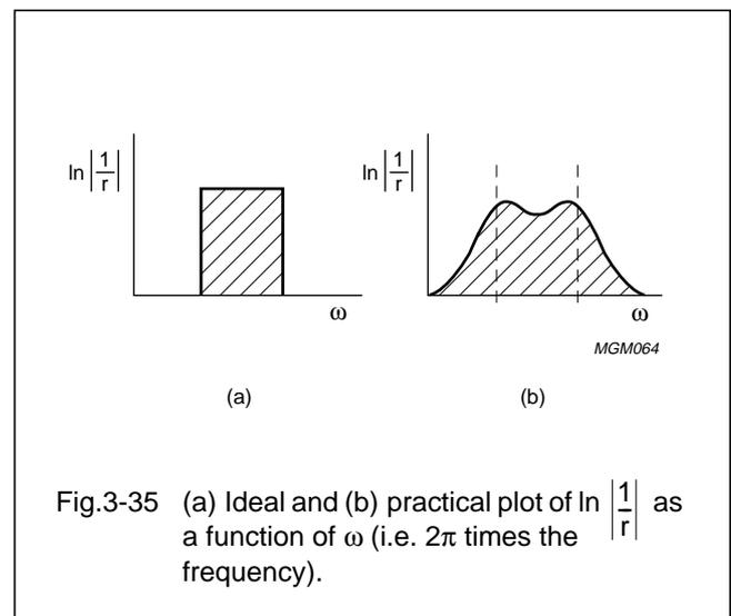
Fig.3-35 (a) Ideal and (b) practical plot of  $\ln \left| \frac{1}{r} \right|$  as a function of  $\omega$  (i.e.  $2\pi$  times the frequency).
