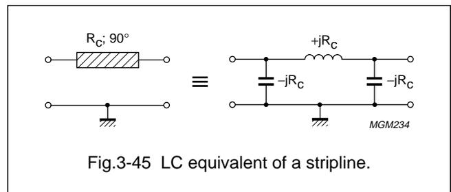
Fig.3-45 LC equivalent of a stripline.
