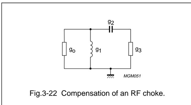
Fig.3-22 Compensation of an RF choke.
