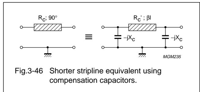
Fig.3-46 Shorter stripline equivalent using compensation capacitors.
