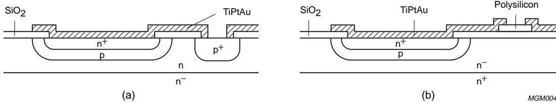
Fig.1-6 Emitter resistance formed (a) by a p<sup>+</sup>-diffusion beside the base areas, and (b) as a doped polysilicon layer on top of the oxide.
